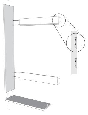
Rest the fiberglass panel into the back of the frame.
