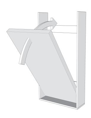
Guide the other side section onto the dowels and secure with two large flush-mount Phillips screws from below.
