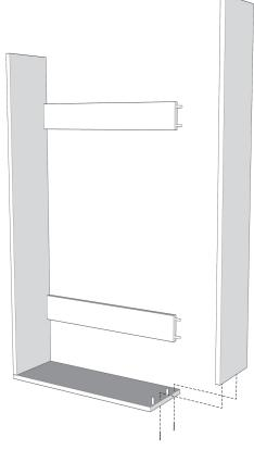
Insert two wooden dowels into the bottom section for the center divider.
