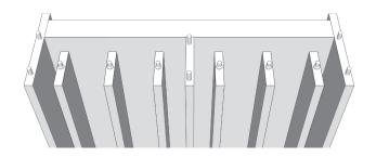
If the vertical deflectors are to be fixed in place insert a second metal pin in the rear hole of each deflector. Skip this step if the deflectors are to be movable and continue to step-8.
