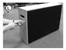
When dry, remove the protective plastic and re-insert panels. Secure the panels in place with the eight large screws [9] using the pre-drilled holes in the sides.
