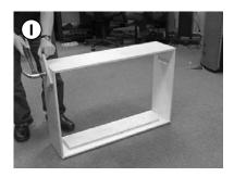
Add glue to the joints and tap flush. Follow the glue manufacturer's instructions for dry times.
