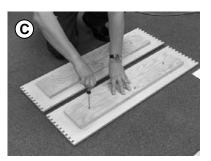
Attach the panel stops [3] to the top and bottom pieces [2]. Drive three medium screws [8] into the pre-drilled holes in the top and bottom. These will be used to hold the springboard and position the acoustic panels.
