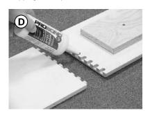
You are now ready to glue the first section of the Go-Trap together. A few drops of wood glue in the dovetail joints is all you need. Use a drop cloth to prevent excess glue from making a mess.
