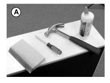
Collect your tools and materials. You will need a piece of scrap wood to protect the finish when tapping the parts together. When working with glue, it's a good idea to lay down a drop cloth or use the shipping box to protect the floor.
