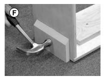
Using a piece of scrap wood, tap the joint together with a hammer until flush. The scrap wood will protect the finish from tool marks. Wipe away excess glue that is forced out of the joints.
