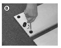
There are four pre-drilled holes in the bottom piece [2]. Install the four rubber feet [6] into the bottom piece using the small screws [7].
